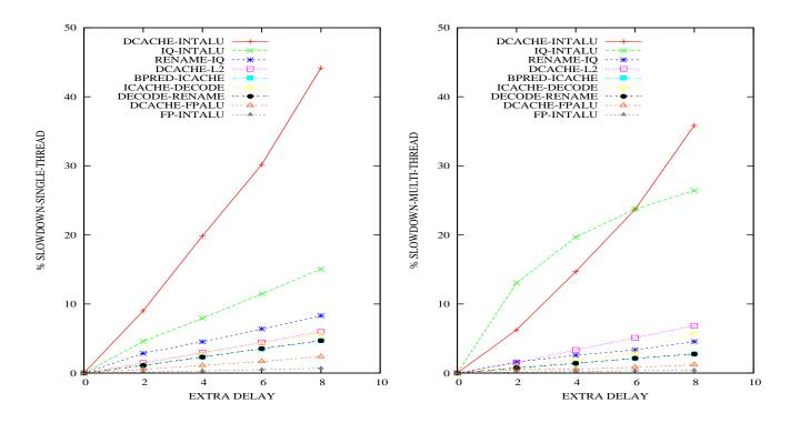
Figure 2: IPC slow-down curves for single-threaded and multi-threaded workloads.
