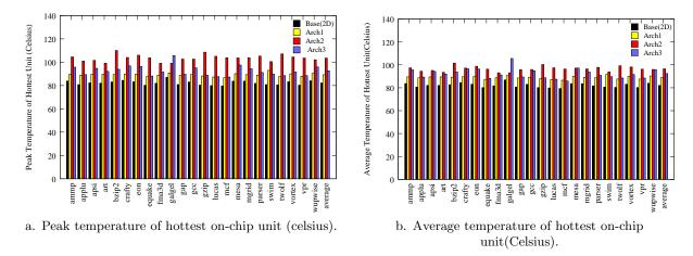
Figure 8: Peak and Average Temperatures of hottest on-chip structures.
