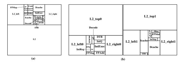
Figure 3: Optimal 2D and 3D floorplans.
