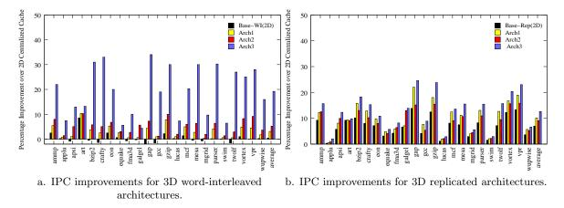
Figure 7: 3D clustered architectures, relative to a 2D organization with a centralized cache.
