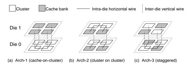
Figure 6: Block diagrams for 3D organizations of the 4 cluster system.
