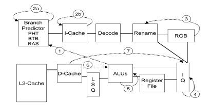
Figure 1: Critical microarchitecture loops in an out-of-order superscalar pipeline.
