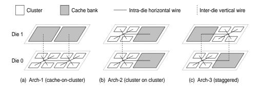
Figure 5: Block diagrams for 3D organizations of the 8 cluster system.
