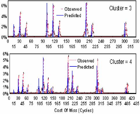
Figure 14: Observed and predicted Spectrogram for Clusters = 3 and 4. L1=64KB, L2=256KB, 15 cycle latency, L3 = 100 cycle latency.
