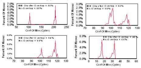
Figure 8: Cluster Size = 2 Individual Miss Spectrograms, L1=64KB, L2=256KB, 15 cycle latency, L3 = 100 cycle latency, OLTP.
