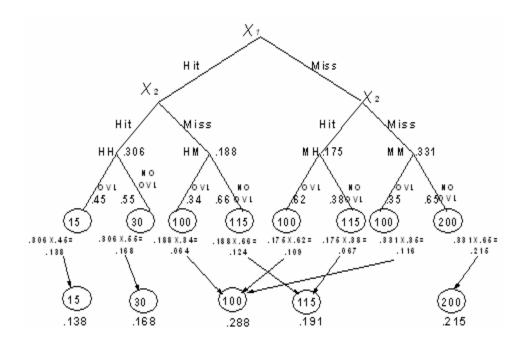
Figure 9: Miss Spectrogram Construction. HH, MM, HM, MH, and overlap probabilities for Cluster = 2 Spectrogram. Data is for the OLTP workload.
