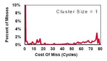
Figure 23: Instruction Spectrogram Data for the OLTP workload.
