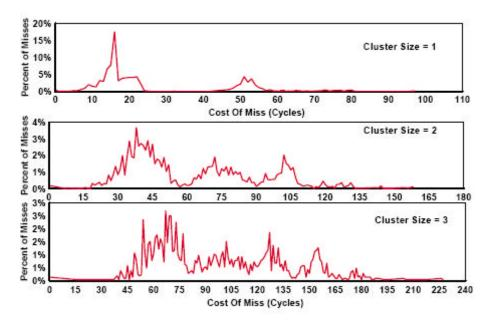
Figure 24: Data Miss Spectrogram. L1=64KB, L2=256KB with 15 cycle latency, L3=50 cycles latency. Line Transfer = 16 Cycles.
