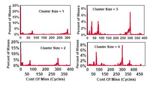
Figure 22: Instruction Miss Spectrogram. L1=64KB, L2=256KB with 15 cycle latency, L3=1MB with 75 cycle latency, and memory with 300 cycle latency.
