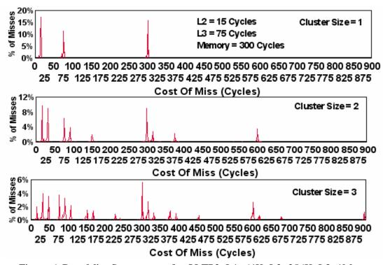
Figure 6: Data Miss Spectrogram for OLTP2, L1=64K, L2=256K, L3=1Meg.
