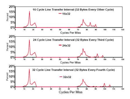
Figure 15: Cluster = 1 Miss Spectrogram for OLTP3 for 16, 24, and 32 cycle trailing edge.
