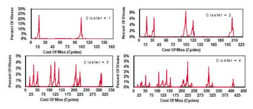
Figure 3: Miss Spectrogram for OLTP, L1 = 64K, L2 = 256K, Infinite L3; 15-cycle L2, 100-cycle L3.
