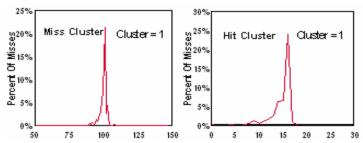
Figure 7: Individual Miss Spectrogram for Cluster Size = 1, L1=64KB, L2=256KB, 15 cycle latency for L2 Hit, L3 = 100 cycle latency for L2 Miss, Data for OLTP.
