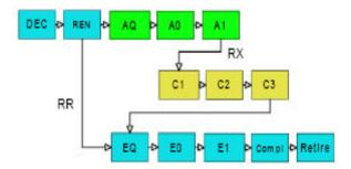
Figure 2: Pipeline modeled for study. Stages include: Decode, Rename, Agen Q, Agen, Cache Access, Execute Q, Execute, Completion, and Retire.
